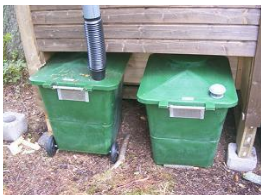
Figure 14. Movable ventilated collecting bins with overflow for leachate discharge (source: PikkuVihreä, Finland).
